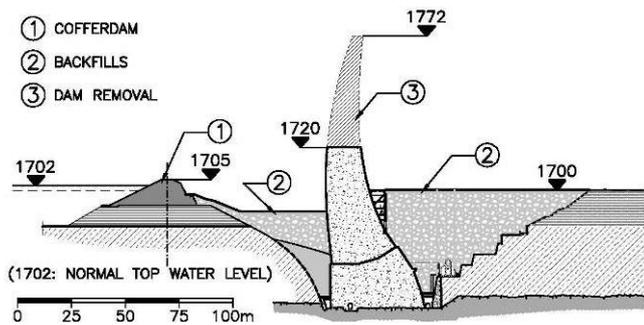
Figure 9: Storage of the material demolition
